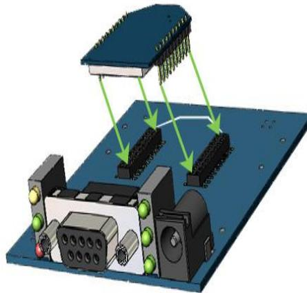
**Figure 1: Zigbee Module Mounting to an RS232 Interface Board.**
