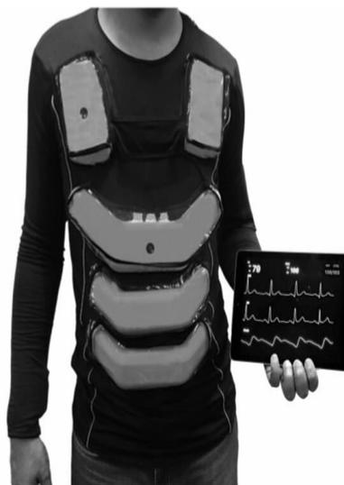
Prototype of wearable vital signs monitor.
