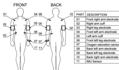
Fig. 1. Scheme of sensors distribution around the body used in the vital signs monitor.
